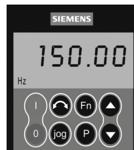
Fig. 15 — Siemens VFD Low Ambient Temperature Controller
